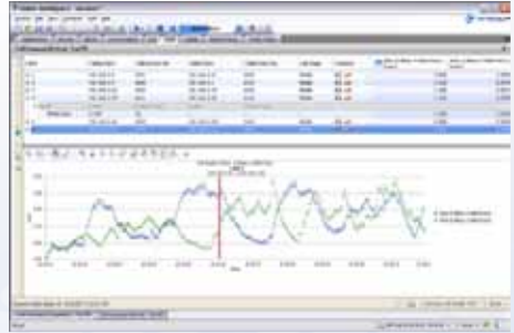
VoIP conversations are easily graphed to visualize voice impairments. Audio playback is also included.
